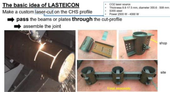
Figure 1 Laser cutting techniques, machine and approach to develop the LASTEICON and LASTTS joints. [9]
